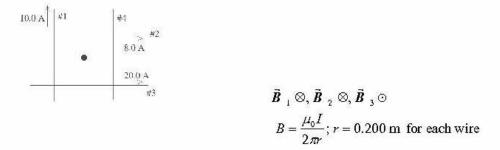
$B_1 = 1.00 \times 10^{-5} \text{ T}, B_2 = 0.80 \times 10^{-5} \text{ T}, B_3 = 2.00 \times 10^{-5} \text{ T}$ Let  $\odot$  be the positive z-direction.  $I_1 = 10.0 \text{ A}, I_2 = 8.0 \text{ A}, I_3 = 20.0 \text{ A}$  $B_{1z} = -1.00 \times 10^{-5} \text{ T}, B_{2z} = -0.80 \times 10^{-5} \text{ T}, B_{3z} = +2.00 \times 10^{-5} \text{ T}$  $B_{1z} + B_{2z} + B_{3z} + B_{4z} = 0$  $B_{4z} = -(B_{1z} + B_{2z} + B_{3z}) = -2.0 \times 10^{-6} \text{ T}$
